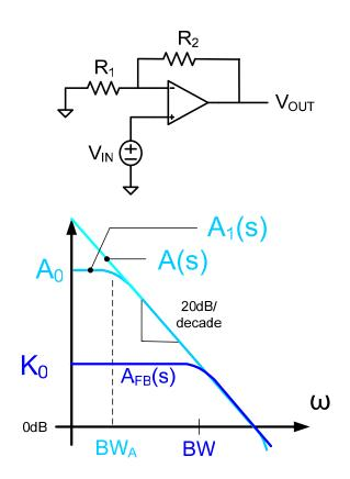
Problem 2 Determine the 3dB bandwidth of the following circuits if the op amp is the National LMP 2231 biased with a single 5V dc power supply.
