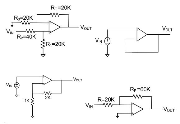
Problem 3 Determine the 3dB bandwidth of the cascade of 4 identical noninverting amplifiers and compare with that of a single noninverting amplifier if both structures are to achieve the same gain. Assume all op amps have a gain bandwidth product of GB.
